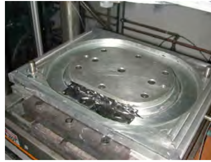
Lay-in L-shaped Front and Back Rib Plies
