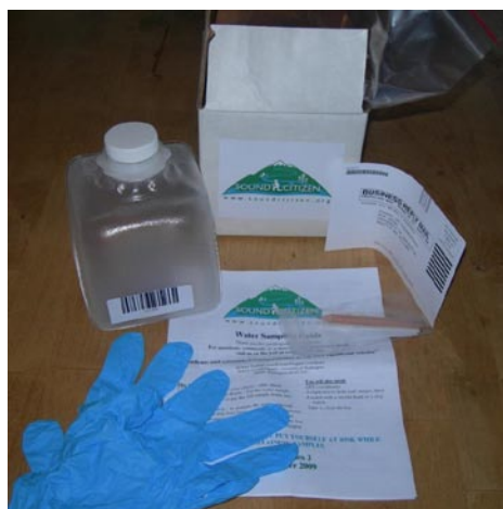
Figure 2. A typical SoundCitizen sampling kit sent by mail to volunteers. Kits contain an instruction sheet and pencil, a pre-cleaned sample bottle with barcode, gloves, chemical test strip for evaluating water prior to mailing, and a pre-paid mailing label to assist in returning the sample to the university.
