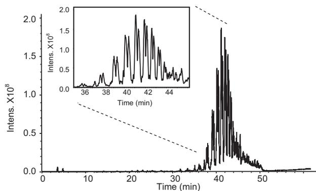
**Figure 1.** LC/ESI-MS base peak chromatogram of a mixture of non-methylated linear polypropyleneimine standards (LCPA mixture A). The top insert shows a close-up of the LCPA elution time window (RT = 36–46 min).
