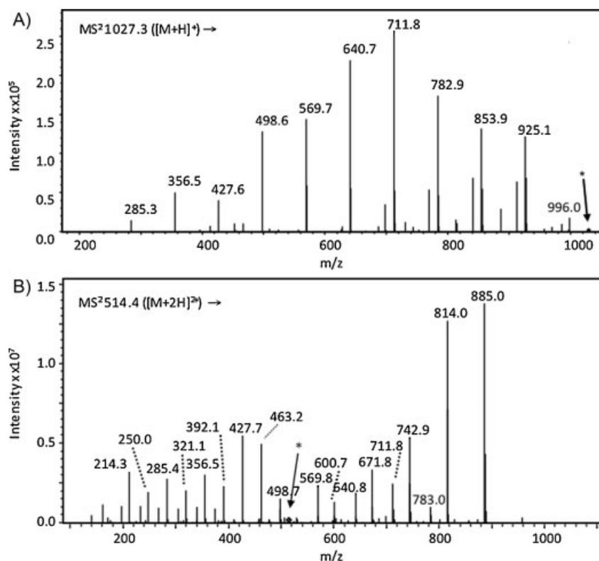
**Figure 9.** LC/ESI-MS/MS product ion mass spectra of the protonated singly (A) and doubly (B) charged molecular ion of LCPA peak # 12' (LCPA standard mixture B;  $m/z$  1026.3).
