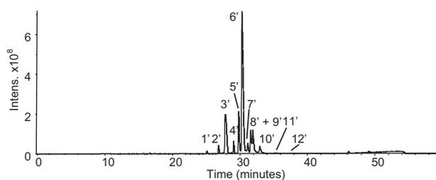
**Figure 3.** LC/ESI-MS base peak chromatogram of a mixture of methylated, linear polypropyleneimine standards (LCPA mixture B). The top shaded inset displays the general structure of the compounds present in the mixture. Refer to Table 2 for peak assignment.
