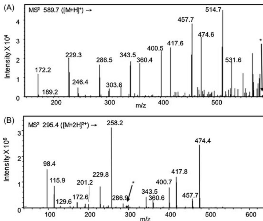
**Figure 7.** LC/ESI-MS/MS product ion mass spectra of the protonated singly (A) and doubly (B) charged molecular ion of LCPA peak # 6 (LCPA standard mixture A;  $m/z$  588.7).
