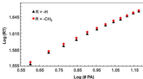
**Figure 4.** Log-log plot of retention times (RT, in minutes) versus number of propylamine repeat units (#PA) for non-methylated ( $R = -H$ ) and partially methylated ( $R = -CH_3$ ) long-chain polyamines from the standard mixture A (see general structure in Fig. 2).
