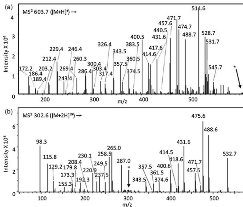
**Figure 8.** LC/ESI-MS/MS product ion mass spectra of the protonated singly (A) and doubly (B) charged molecular ion of LCPA peak # 18 (LCPA standard mixture A;  $m/z$  602.7).
