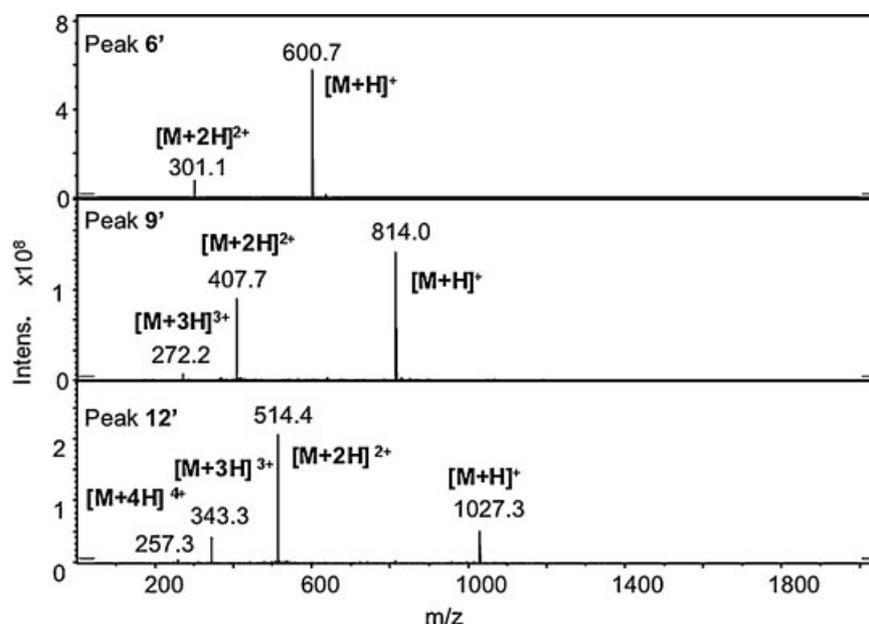
Figure 6. LC/ESI-MS spectra of selected LCPAs from standard mixture B (see chromatogram in Fig. 3).
