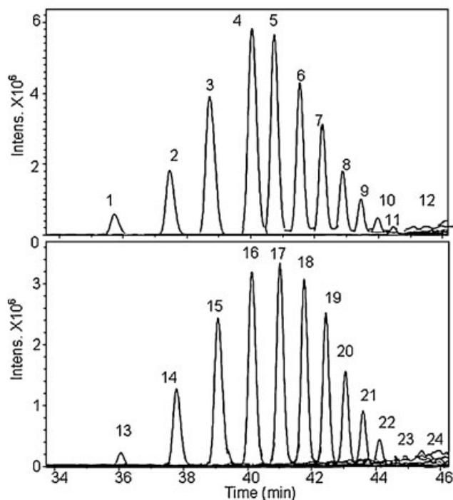
**Figure 2.** Overlapped LC/ESI-MS extracted ion chromatograms of LCPA standard mixture A, containing non-methylated LCPAs (peaks 1–12,  $n=4-15$ ;  $R=H$ ) and partially methylated LCPAs (peaks 13–24,  $n=4-15$ ;  $R=-CH_3$ ). The top shaded inset displays the general structure of the compounds present in the mixture. Refer to Table 1 for peak assignments.
