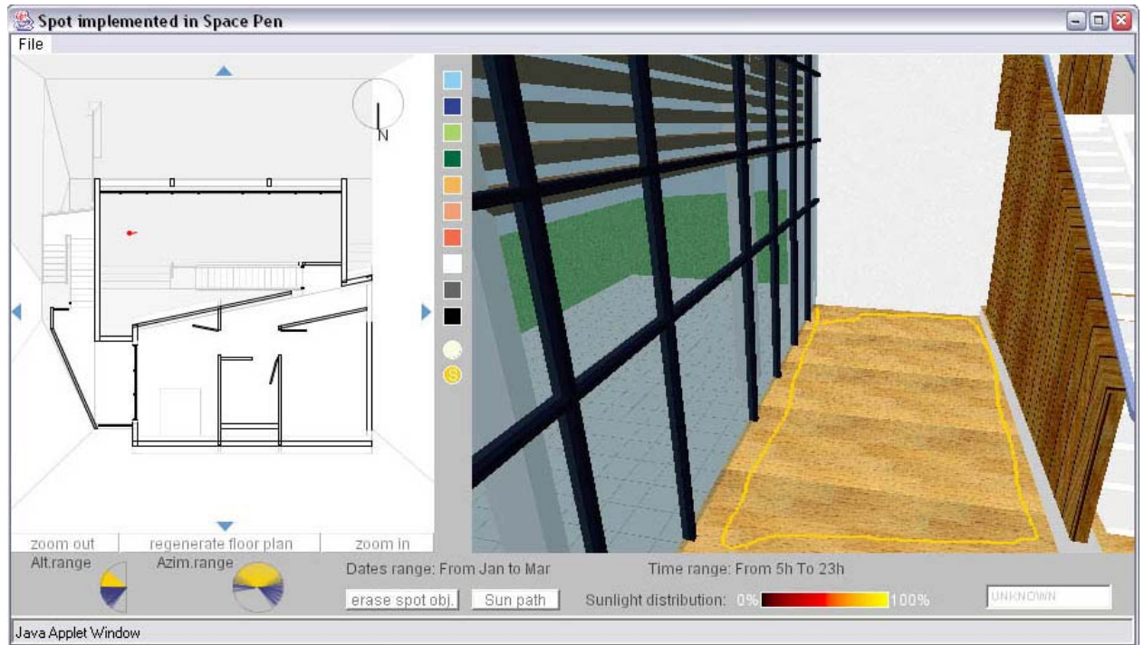
(Fig 7.3): Selecting an area for simulation by drawing on the 3D model.
