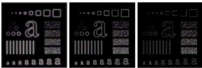
FIGURE 4.26 Results of highpass filtering the image of Fig. 4.11(a) using a GHPF of order 2 with D_0 = 15, 30, and 80, respectively. Compare with Figs. 4.24 and 4.25.
