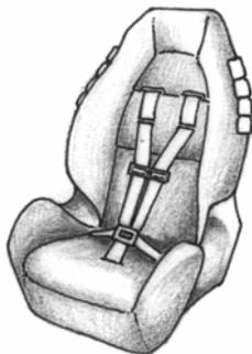
**Shield booster:** Using the shield portion of this booster is no longer advised. If the shield comes off, take it off (check instruction book). Then use the booster seat with the lap/shoulder style seat belt for children over 40 pounds. It works like a no-back booster seat. This style works best in cars with headrests.
