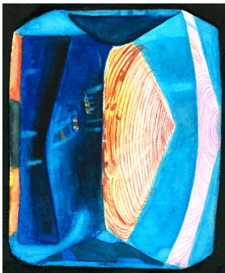
Fig. 4 Water painting of a crystal of K_2SO_4 (width ca. 1 cm) grown in the presence of ortho -aminobenzene sulfonate. The blue luminescence of the benzene derivative from the (021) sector is excited with ultraviolet light. Additionally, a visible light was reflected from the rightmost face. The pattern of light results from the selective staining of macro-growth spirals. See photograph by R. W. Gurney in ref. 7.
