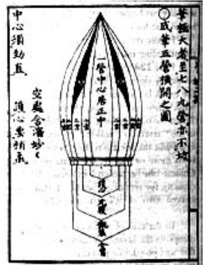
Drawing of cross-section, internal structure of brush
