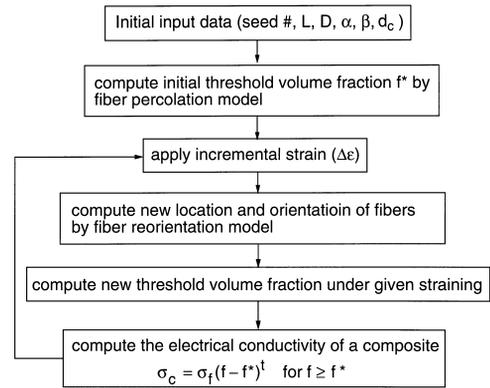
Fig. 7. The computation procedure of the present model.
