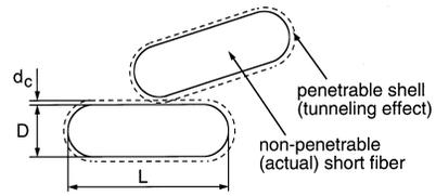
Fig. 3. The simulation of non-penetrable model ( $D$  = actual fiber diameter,  $d_c$  = tunneling distance).
