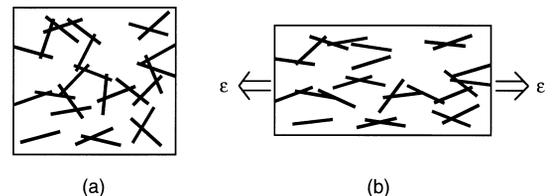
Fig. 1. The expected microstructure change of a composite under straining; (a) percolating before straining (electrically conductive) and (b) non-percolating after straining (non-conductive).
