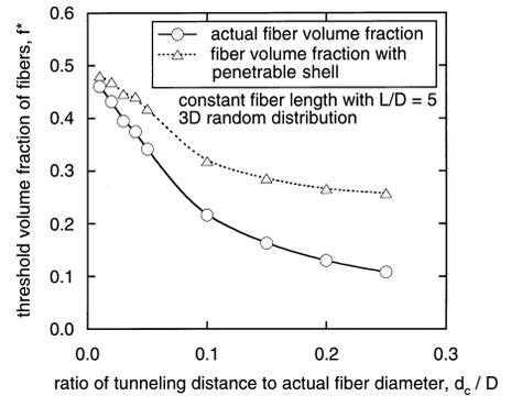
Fig. 5. The threshold volume fractions of actual (circles with solid line) and overall (triangles with dotted line) fibers as a function of the ratio of tunneling distance ( $d_c$ ) to actual fiber diameter ( $D$ ).
