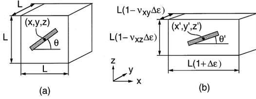
Fig. 4. The 3D fiber reorientation model where only angle  $\theta$  is shown for illustrative purpose; (a) before straining and (b) after straining.
