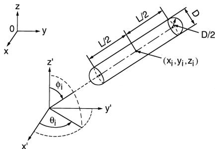
Fig. 2. A capped cylindrical fiber in a 3D space.
