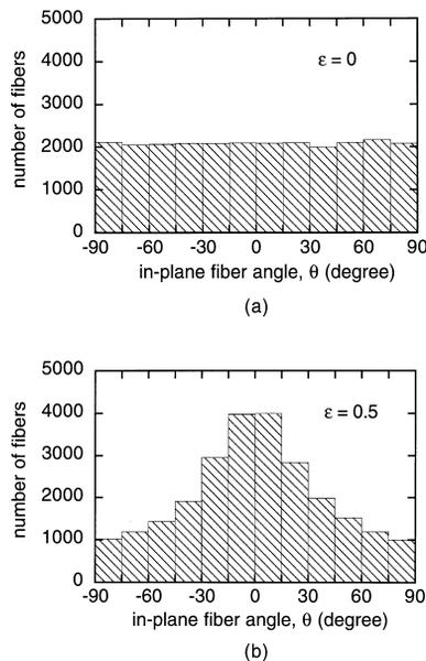
Fig. 6. The reorientation of fibers under straining of an isotropic composite (total number of fibers = 25,000); (a) before straining ( $\varepsilon = 0$ ) and (b) after straining ( $\varepsilon = 0.5$ );  $L/D = 55$ .
