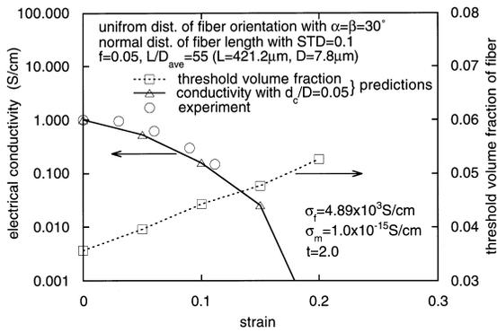
Fig. 8. The electrical conductivity of a composite and threshold volume fraction of conductive fiber as a function of the applied strain.
