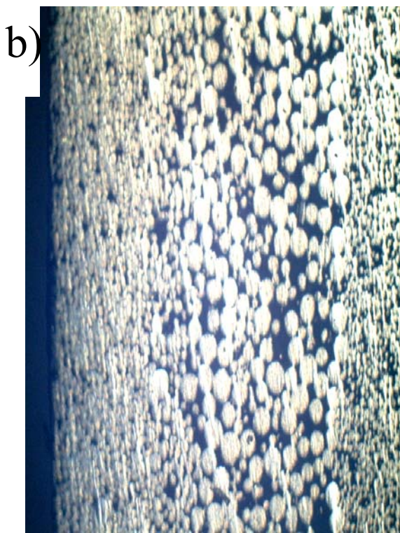
Porous graded porous structure of NiTi a) 750 °C b) 850 °C c) 950 °C
