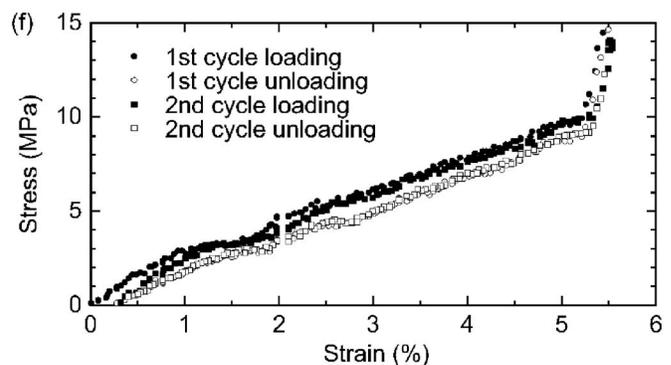
FIG. 4. [(a)–(e)] Change of volume ratio of CVs for the first loading and (f) stress-strain curves for the first two cycles of loading and unloading.
