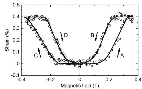
FIG. 3. Magnetic field-induced strain as a function of magnetic flux density measured in Fe-Pd single crystal. The magnetic flux density was increased and decreased in alphabetical order.
