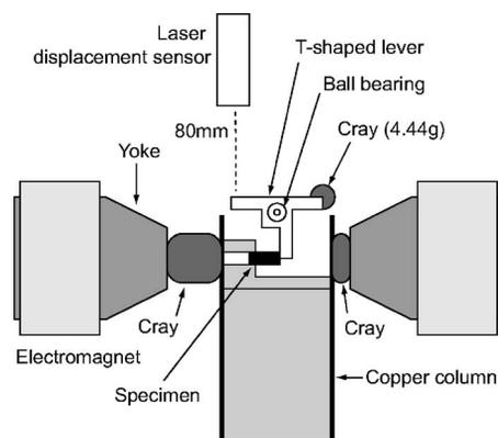
FIG. 1. Experimental setup for magnetic field-induced strain measurement.
