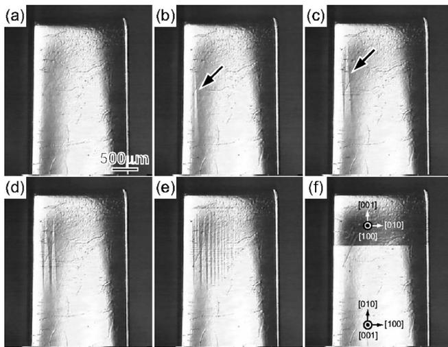
FIG. 2. Surface morphology change of the single crystal specimen during martensitic transformation. The arrows indicate growing wedge-shaped HPVs. The crystallographic orientations of the two fct martensite variants are shown in (f).
