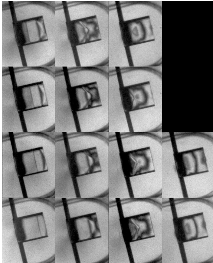
Figure 9.7: Laboratory experiment where a shock wave propagates through an acrylic cylinder and the stresses are photographed using a high speed camera and polarized filters[30]. Courtesy of Dr. Michael Bailey's group in the University of Washington Applied Physics Lab.
