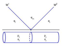
Left-going wave  $W^1 = q_m - q_l$  and right-going wave  $W^2 = q_r - q_m$  are eigenvectors of A.
