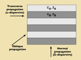
Dispersion of normally-propagating waves is caused by **reflection** and depends on **impedance** variation (Z-dispersion)
