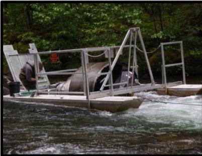
Collecting smolt data using a rotary smolt trap
