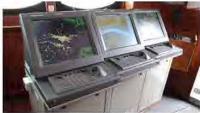
Figure 2: The ECDIS is a cyber-dependent system installed on the bridge of a vessel as a supplement—or often a replacement—of paper chart navigation.
