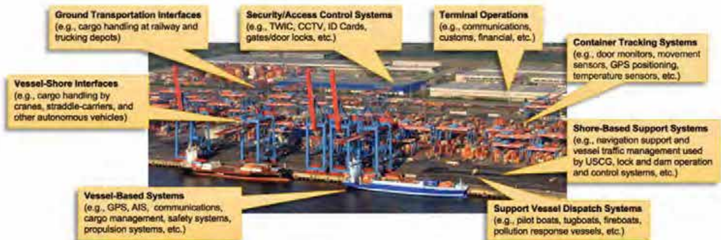
Figure 1: A selection of the interacting cyber-dependent systems and components found at a typical maritime shipping port. Photo Credit: Ajepbah [CC-BY-SA-3.0 DE], via Wikimedia Commons
