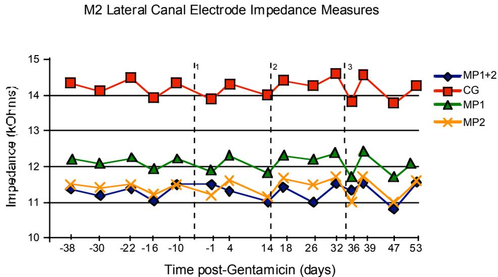
Figure 6. Longitudinal changes in electrode impedance measured in the most distal lateral canal electrode in a single rhesus monkey. Several return configurations are displayed.
