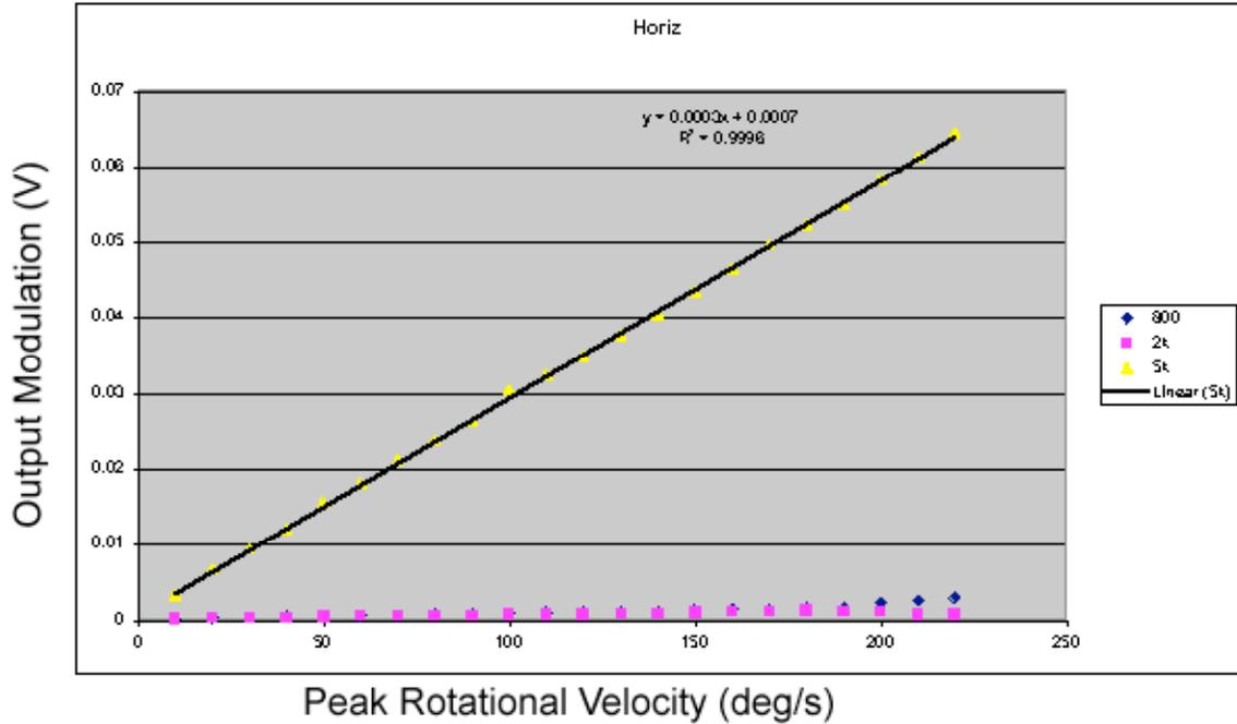
Figure 1. Amplitude modulation versus peak rotational velocity for each of the carrier frequencies in the audio output of the bone anchored sensory array during head rotation in the lateral canal plane, corresponding to the 5Khz carrier.
