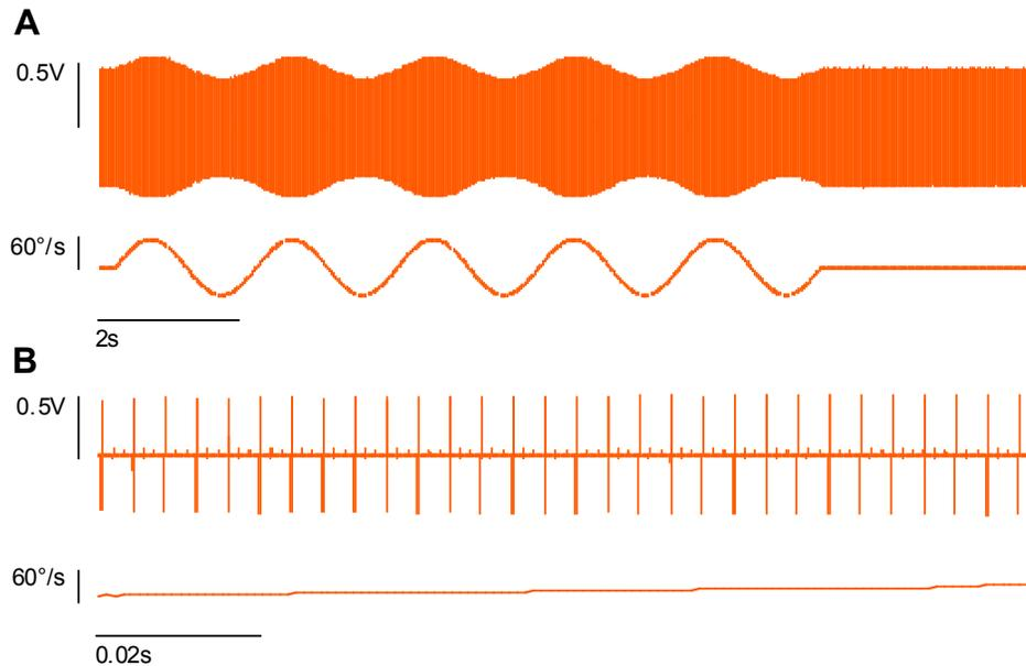
*Figure 3. Response of the bone anchored sensor array to sinusoidal rotation in the plane of the right lateral canal. A: Current modulation of one stimulating electrode (channel E6, upper trace) during rotation of the bone anchored vestibular processor in the lateral canal plane (chair tachometer, lower trace). B: Detail showing individual stimulating pulses (channel E6, upper trace) and the chair tachometer output (lower trace) with an expanded time scale.*
