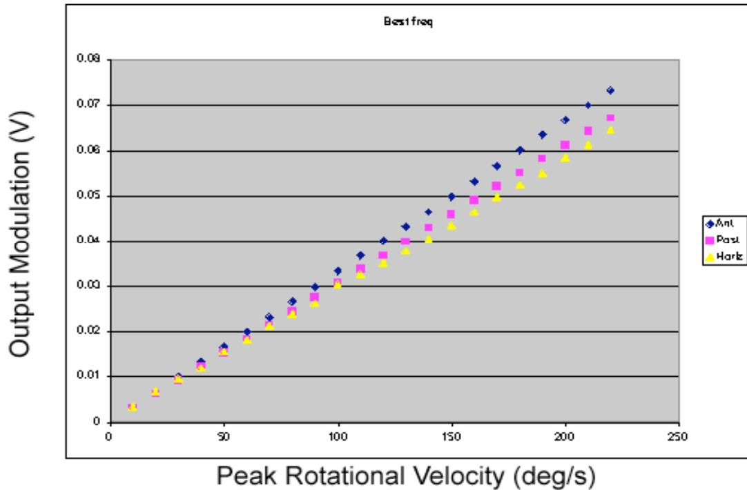
Figure 2. Amplitude modulation versus peak rotational velocity for each of the carrier frequencies in the audio output of the bone anchored sensory array during head rotation in the optimal plane for each carrier.
