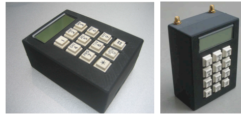
Figure 7 Prototype of the *box. Note the golden pigtail connectors on the top of the box to allow easy attachment of GSM and GPS antennas.
