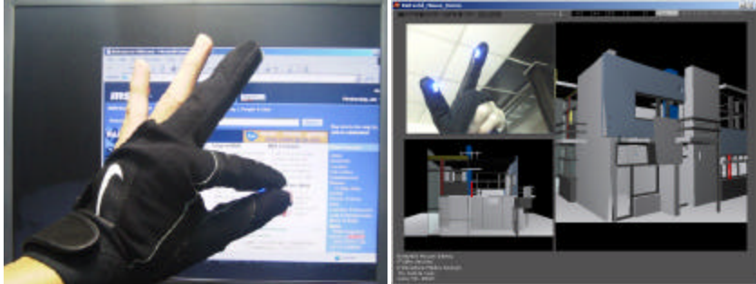
Figure 4. The presenter puts on LED-mounted half-finger gloves and uses hand gestures to point, grasp, and move digital contents (on the left); Specific hand gestures control the viewpoint of a digital model (on the right).
