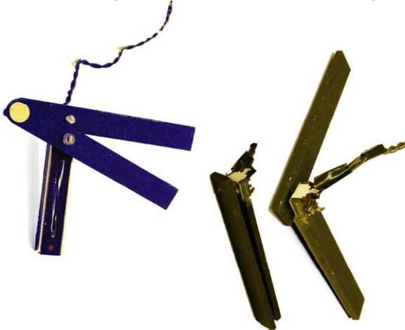
Figure 8: Left: sliding potentiometer measures angle; right: rotational potentiometer makes and measures hinge.
