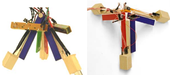
Figure 7: Popsicle-stick hub with sliding (left) and rotational (right) potentiometers to measure angle.
