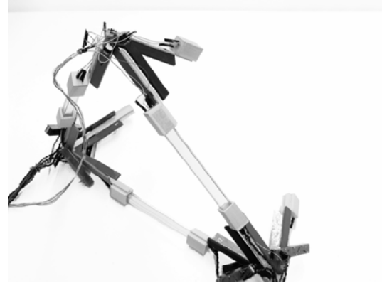
Figure 6: Clear acrylic struts connect three hubs.
