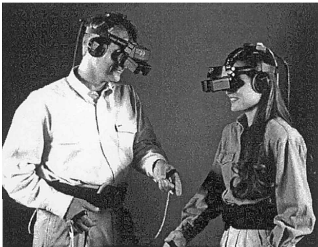
Figure 9. Users wear “VR gear” consisting of HMD, position trackers, and microphone, which immerses them in the virtual world.
