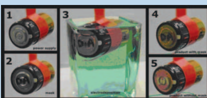
It illustrates how a simple battery can demonstrate electrodeposition.
