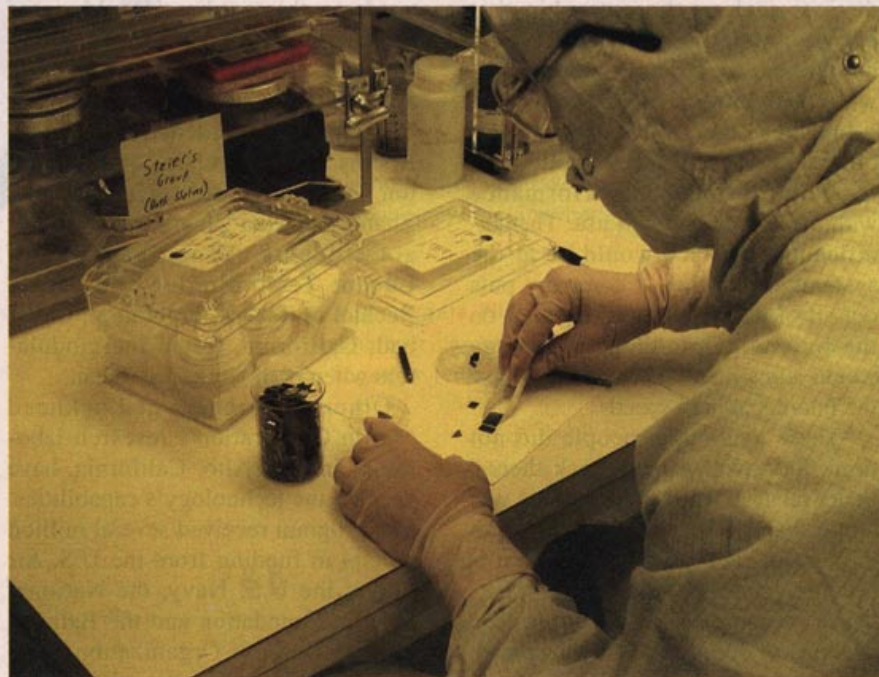
Min-Cheol Oh, University of Southern California (USC) research associate in electrical engineering/electrophysics, works with recently developed polymeric electro-optic chips in the university clean room. These new chips have the potential to eliminate bottlenecks in optical links, which would vastly increase bandwidth over fiber.
