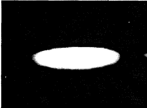
Fig. 3 The near field pattern of a single mode buried channel waveguide made by direct laser writing.
