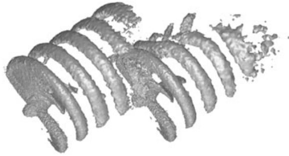
Figure 20. Iso-surfaces of constant vorticity shown with blades at 45° position.
