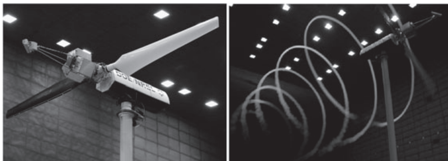
Figure 2. NREL Phase VI rotor in operation during wind tunnel test (from Hand et al. 11 ).
