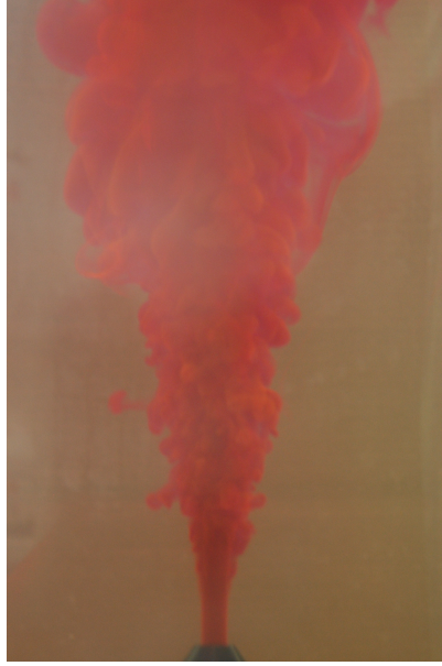
Figure 3.10: Photograph of a Rhodamine-dyed water jet
