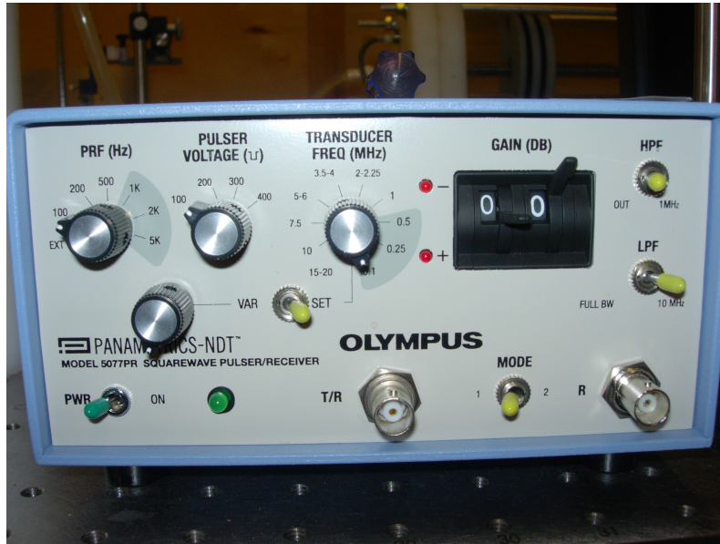
Figure 3.4: Front face of control box that connects the transducer to the NI PCI-5114 card
