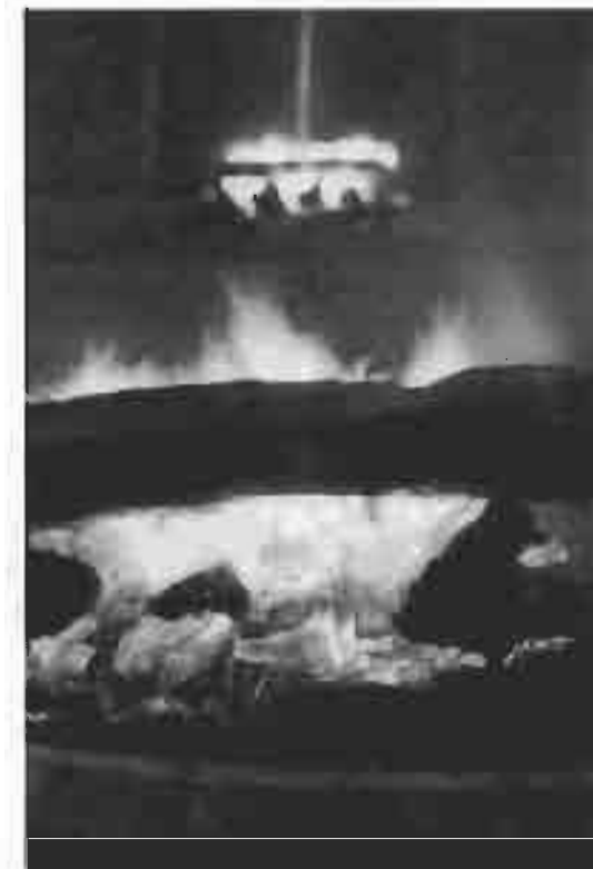
PHOTO 7. Fire over air supply grate
