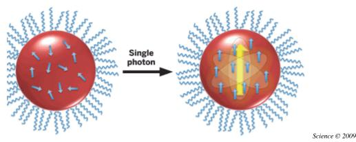
*Exposing this quantum dot to one photon creates an electron-hole pair known as an exciton (yellow arrow), causing manganese impurities (gray arrows) to line up at room temperature.*
