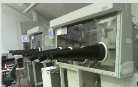
Tandem inert atmosphere system in The Shared Facility for Fabrication and Characterization of Organic Thin Films Thin-Films in Bagley 453.
