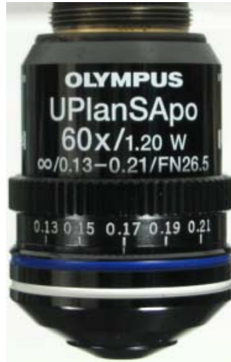
60x/1.2 NA water immersion objective, set at 0.17 (for 0.13 - 0.21 mm thick coverglass)
