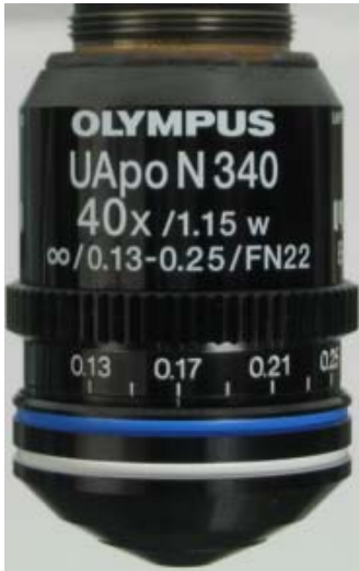
40x/1.15 NA water immersion objective, set at 0.17 (for 0.13 - 0.25 mm thick coverglass)
