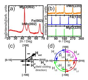
FIG. 1. (Color online) XRD measurements, (a)  $\theta$ - $2\theta$  scan and (b) in-plane  $\Phi$ -scan, of the sample with  $t_{IrMn}$ =14 nm. (c) Geometry of the field cooling direction, magnetic anisotropies, and the external magnetic field. (d) Definition of the various switching fields between different Fe easy axes.
