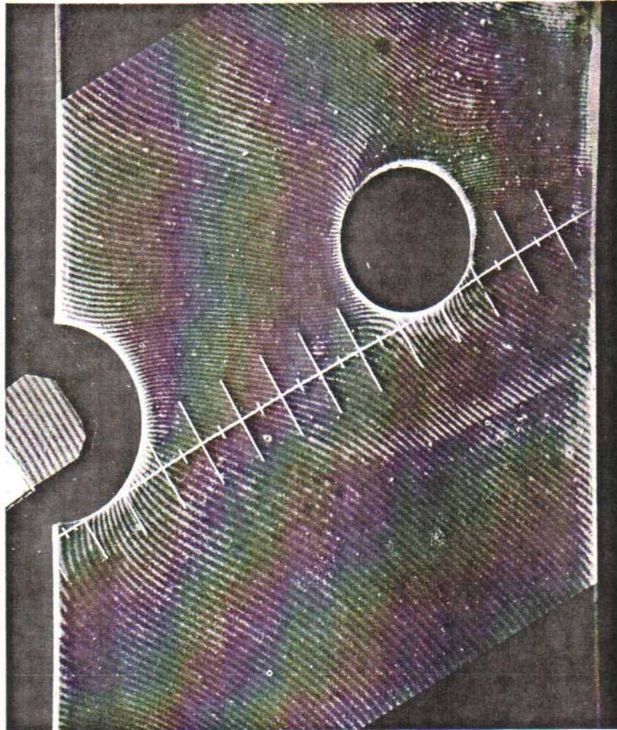
Figure 6-4 Mismatched moiré pattern of displacement components on a rubber specimen ( g = 1/312 in.).
