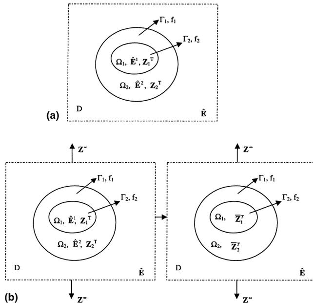
Fig. 4. A double-inhomogeneous-inclusion  $\Omega_1$  and  $\Omega_2$  embedded in an infinite matrix: (a) the double-inhomogeneous-inclusion; (b) the equivalent double-inclusion.
