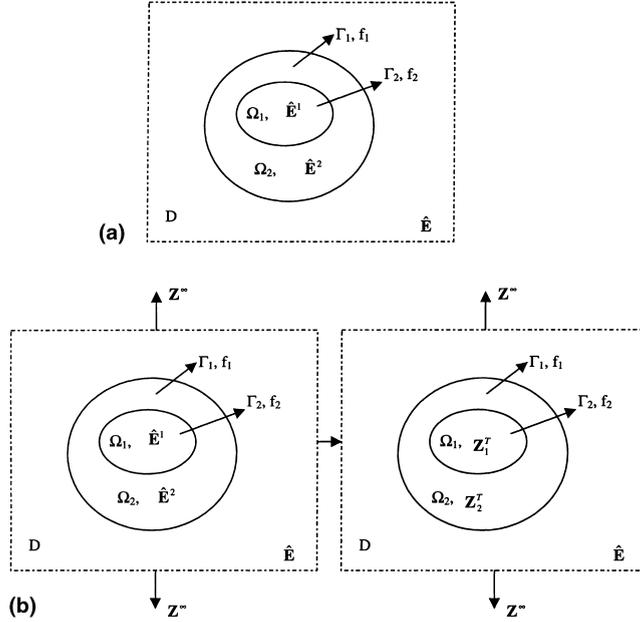
Fig. 3. A double-inhomogeneity  $\Omega_1$  and  $\Omega_2$  embedded in an infinite matrix: (a) the double inhomogeneity; (b) the equivalent double-inclusion.
