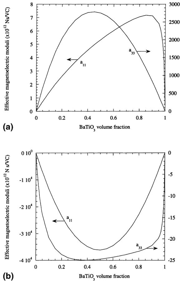
Fig. 5. Magnetoelectric coefficients of piezoelectric-piezomagnetic composites: (a) fibrous composite; (b) laminated composite.
