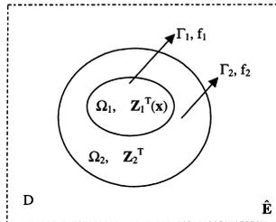
Fig. 2. A double-inclusion  $\Omega_1$  and  $\Omega_2$  embedded in an infinite matrix.
