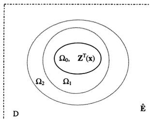
Fig. 1. An inclusion  $\Omega_0$  embedded in an infinite matrix, surrounded by two ellipsoidal surfaces  $\Omega_1$  and  $\Omega_2$ .
