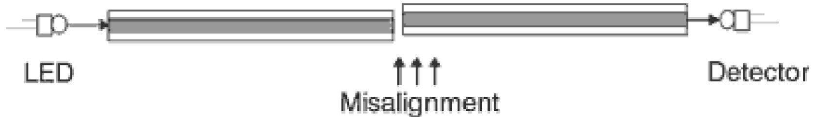
A change in the transverse alignment between two fibers changes the coupling and hence the power falling on the detector.
