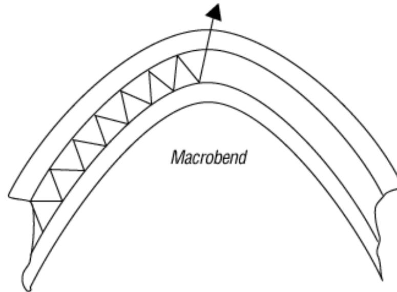
A large-scale bend that is visible; for example, a fiber wrapped around a person's finger. To prevent macrobends, all optical fiber (and optical fiber cable) has a minimum bend radius specification that should not be exceeded.
