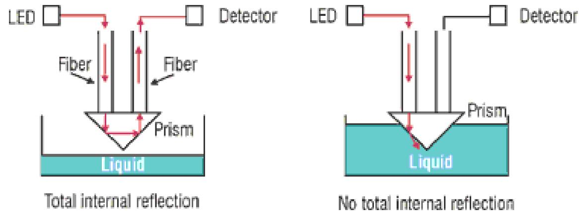
A liquid-level sensor based on changes in the critical angle due to liquid level moving up to contact the sides of the prism (using total internal reflection in air).
