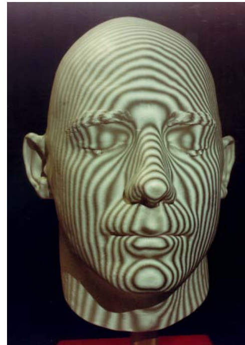
Moiré Fringes Superimposed on Model Head
