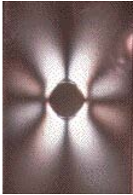
Zero degree isoclinic image for a hole in plate under vertical tension.
