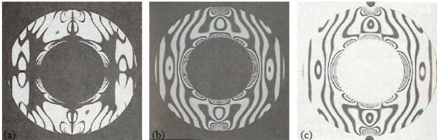
Figure 1: (a) Super-positioning of isochromatic and isoclinic fringes, as seen via a linear polariscope [4]. (b) Isochromatic fringes (lightfield), as seen via a circular polariscope. [5]. (c) Isochromatic fringes (darkfield), as seen via a linear polariscope. [6].
