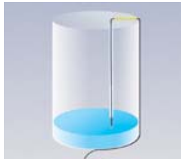
immersion type liquid level detection
