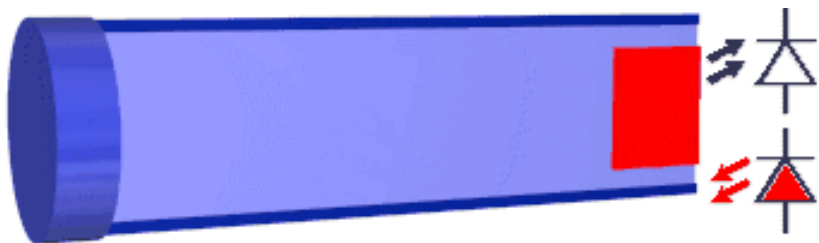
Sensor based on absorbance indicator at solution of different pH
