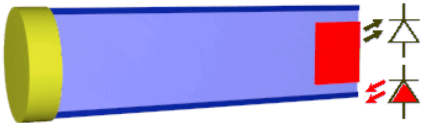
Operating principle of a pH sensor based on absorbance indicator
