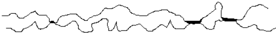
Fig. 3. (a) A representation of two surfaces, rough on small lengthscales, which, when brought into contact (b) show very little actual contact area.
