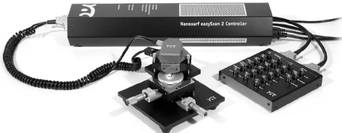
**Easy Scan 2AFM System with optional break-out box**
