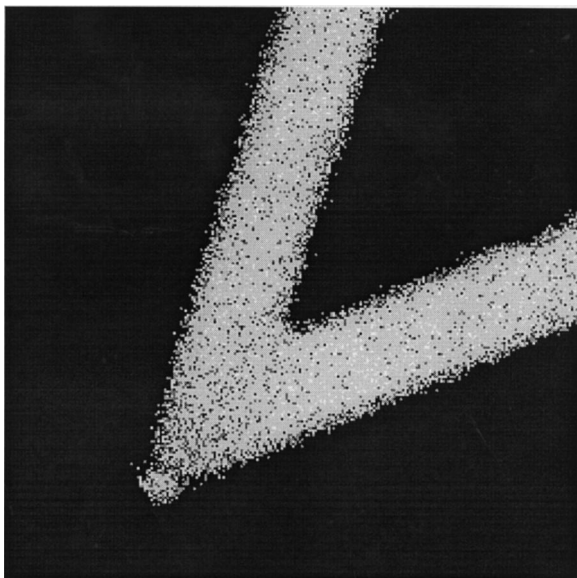
Fig. 4. ToF-SIMS image of a pp-HFP-coated lever. The contrast on the lever was obtained by the detection of C–F ions. No signal from silicon could be detected indicating that the lever was homogenous coated.
