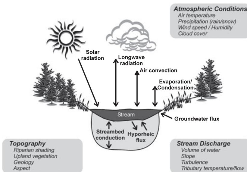
**Fig. 1** Heat exchange processes responsible for variability in water temperatures (bold font) and the physical drivers that control the rate of heat and water delivery to stream and river ecosystems (italic font).
