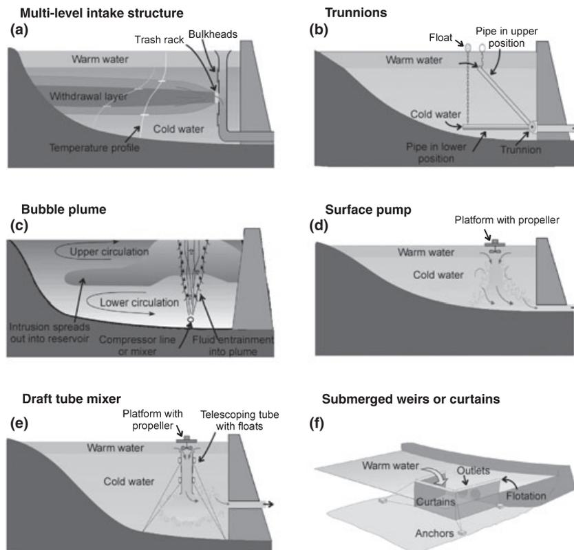
Fig. 5 Current management options for mitigating thermal impacts from dams include: (a) selective withdrawal using multi-level intake structures or (b) trunnions, (c) local destratification using aeration systems, (d) surface pumps or (e) draft tubes and (f) submerged weirs or curtains to redirect either hypolimnetic or epilimnetic water. Figures were provided by Brad Sherman (Australia's Commonwealth Scientific and Industrial Research Organisation: CSIRO).
