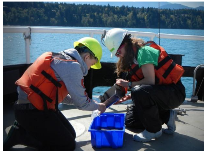
Left: UW professor Chuck Nittrouer and student Sarra Tekola aboard R/V Barnes remove samples from a sediment core taken near the mouth of the Elwha River. Right: Students aboard R/V Barnes retrieve samples of the seabed to be analyzed in the lab. Emily Eidam / UW
