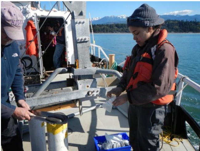
Left: UW professor Chuck Nittrouer and student Sarra Tekola aboard R/V Barnes remove samples from a sediment core taken near the mouth of the Elwha River. Right: Students aboard R/V Barnes retrieve samples of the seabed to be analyzed in the lab. Emily Eidam / UW
