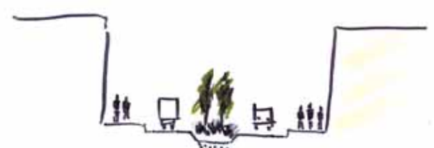
INFILTRATION BOULEVARD TREATMENT
