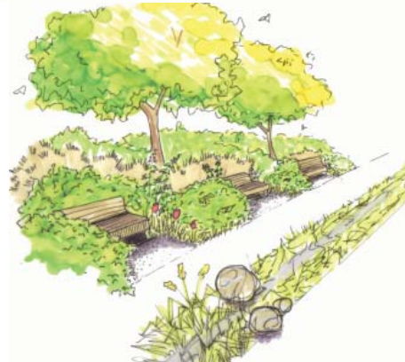
The current sidewalk on NE 100th would be updated to include a vegetated swale where the current grass strip is placed and add benches with vegetation to screen the parking lot below.
