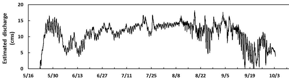
**Figure 10.** *Estimated continuous (hourly) runoff, Jarvis Cr., near the Richardson Hwy in 2013. Note that estimated discharge >14 cms is solely speculative as the measured runoff above > 14 cms was unreliable without a separate depth sounder.*
