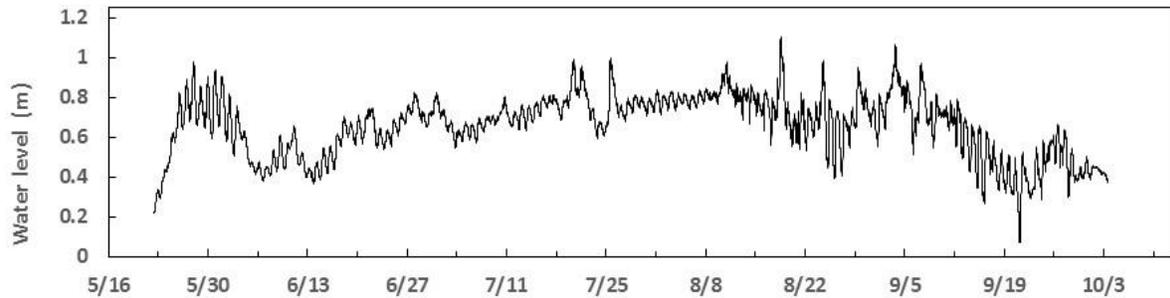
**Figure 8.** Jarvis Cr. 2013 stream water levels (hourly) near the Bridge with the typical diurnal variations.
