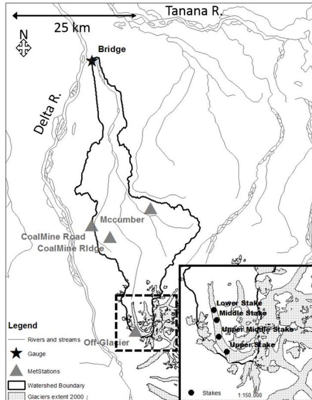
**Figure 1.** Jarvis Cr. watershed boundary with the location of the Bridge runoff measurement site (star) and meteorological stations (triangles). The National Weather Service operated meteorological station is located about 5 km southeast of the runoff monitoring site. Glacier extent as of year 2000 and the mass balance stake locations are presented in the insert.
