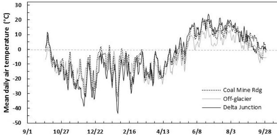
**Figure 3.** Mean daily air temperature during the 2012-2013 hydrologic year at the low- (Delta Junction), mid- (Coal Mine Ridge) and high (Off-glacier) elevation sites.
