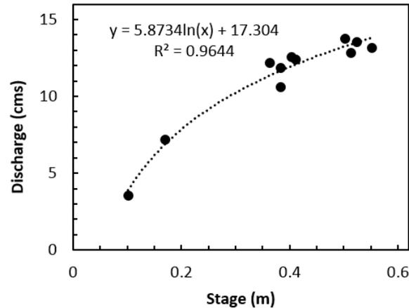
**Figure 9.** Measured discharge (< 14 cms) and coinciding water level during the 2013 season, resulting in a logarithmic stage-discharge relationship.
