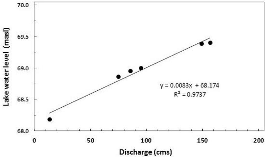
**Figure 14.** Stage-discharge relationship at Valdez Glacier Stream representing the 2012 and 2013 field measurements.
