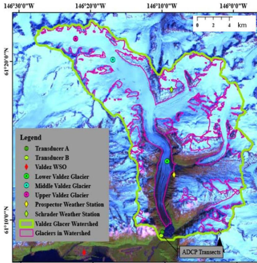
**Figure 2.** Valdez Glacier Stream watershed boundary (green line) with the location of the runoff (“ADCP Transects”) and water level (“Transducer A and B”) measurement sites, meteorological stations including the National Weather Service station in Valdez (“Valdez WSO”).
