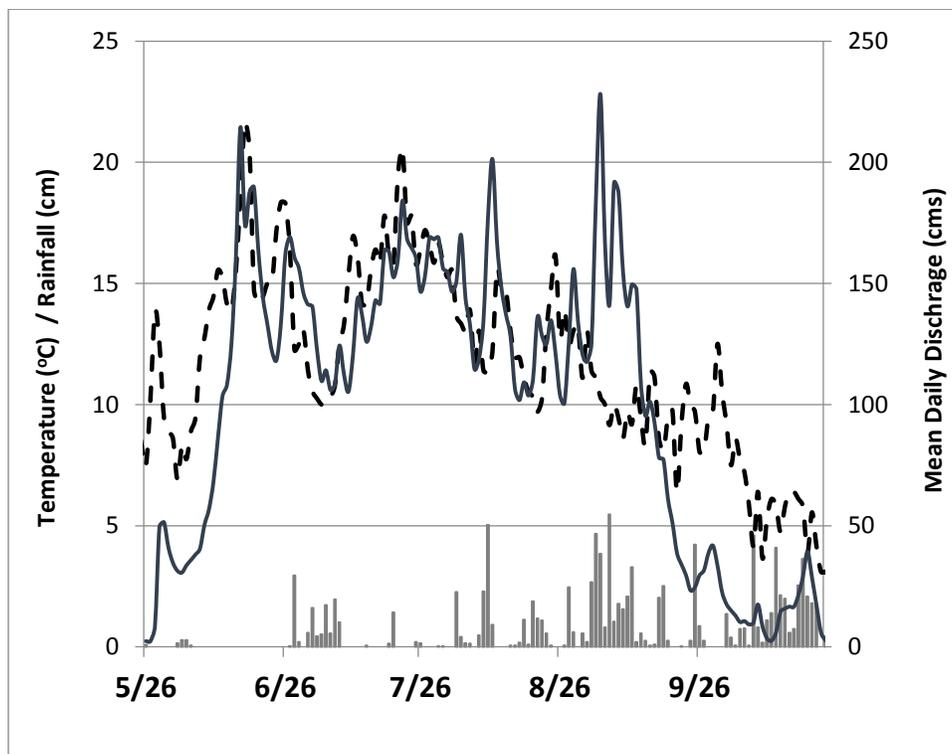
**Figure 15.** Estimated mean daily discharge at the Valdez Glacier Stream during the 2013 melt season (solid line, right axis) and air temperature measured at Valdez WSO (dotted line, left axis). Bar chart shows daily total rainfall events at Valdez WSO (left axis).
