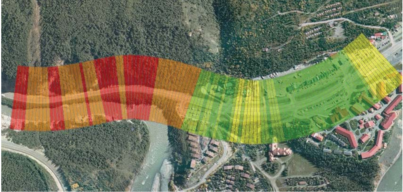
Figure 7.1 Example potential output highlighting areas (10 m sections) along a highway of highest potential landslide or rockfall risk. Note that this figure is based a simple model using only one parameter, slope. The quantitative change analysis results combined with the risk from Phase II will enable us to create much more accurate and reliable highway risk map.
