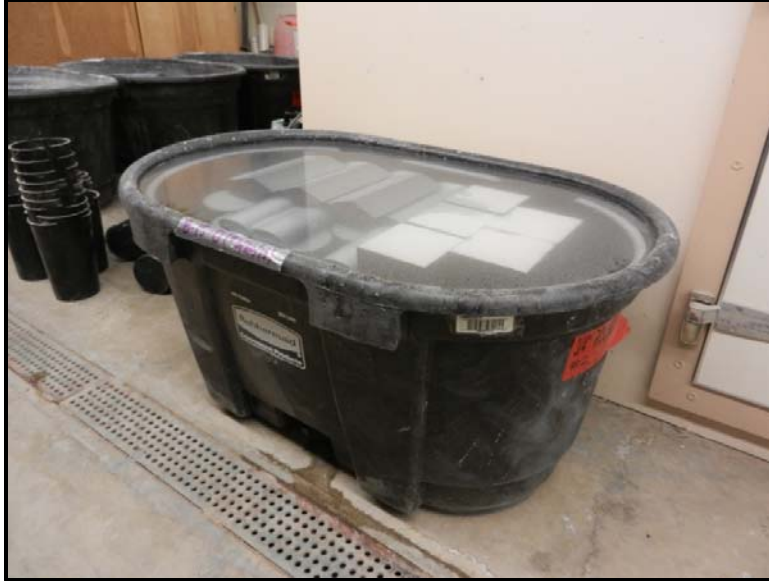
Figure 3.3 Lime-Saturated Water Curing Tub
