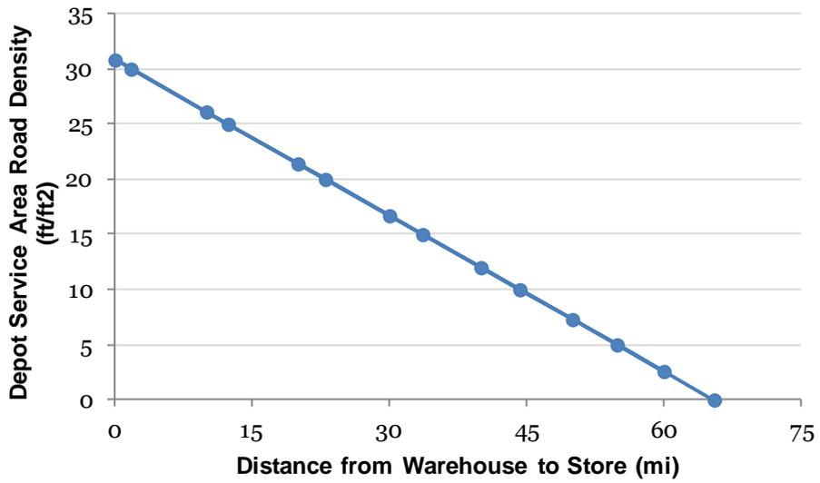
**Figure 5.5** Sensitivity analysis threshold comparing influences on CO2 emissions between passenger vehicles and warehouse delivery goods movement schemes
